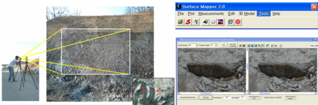
Figure 5. Measuring structural data on rock surface using photogrammetry.
