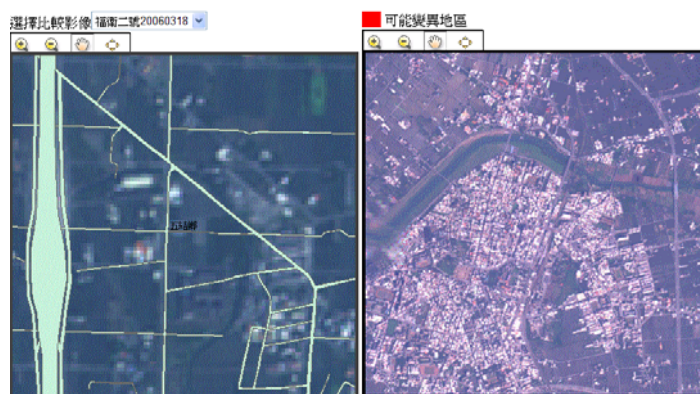
Figure 8. GIS layer overlapping in the demonstration system for land use change surveillance
