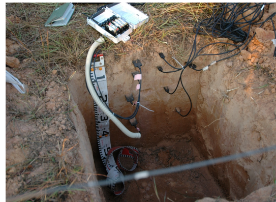
Figure 5. Installation of soil sensors.
